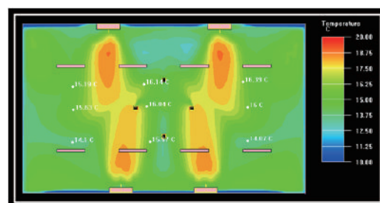
Simulated plane room temperature field distribution in a project
