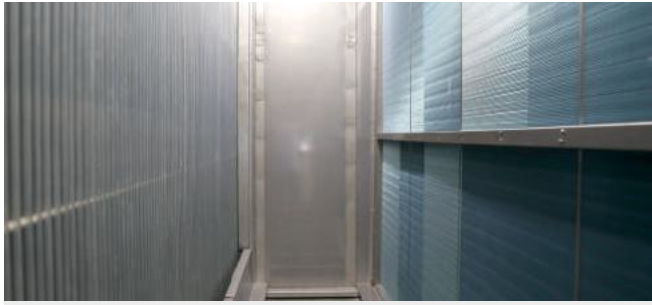
Large-capacity and multi-stage heat exchanger
